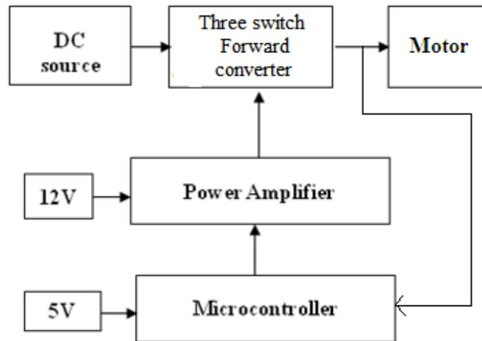
**Fig 1** Block Diagram of Forward Converter system
