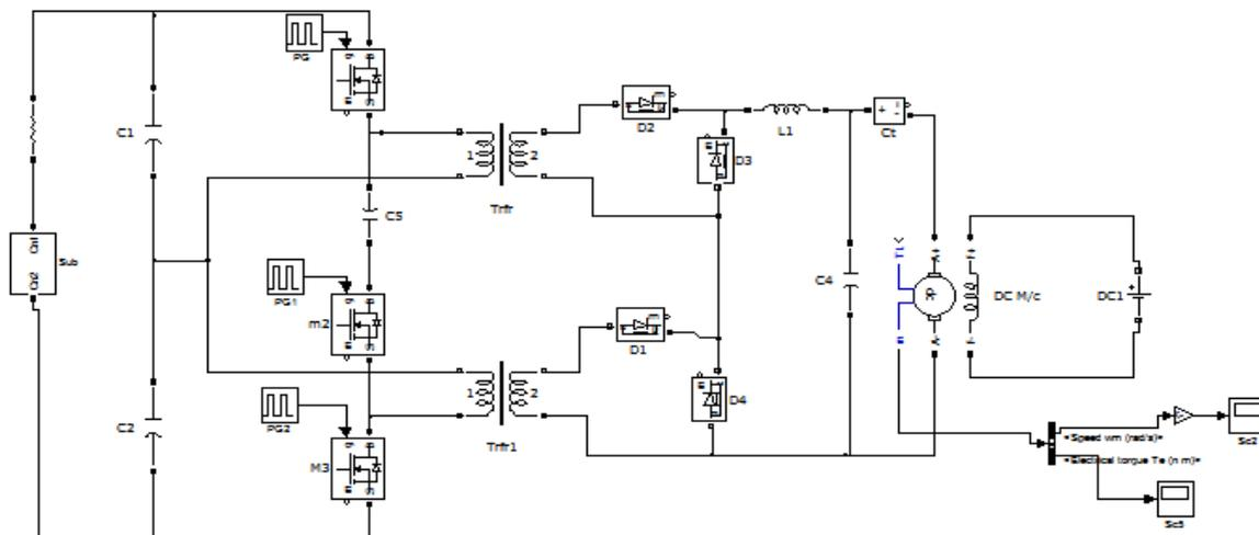
**Fig 2.1** Open loop controlled three switch forward converter with motor load
