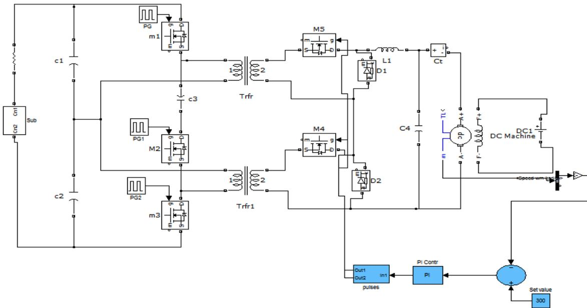
Fig 3.1 Three switch forward converter with closed loop control
